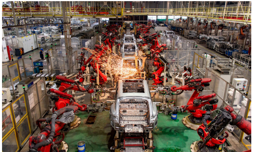
Robotic arms hard at work on a production line in China's Zhejiang Province for the Leapmotor brand of electric vehicles.
